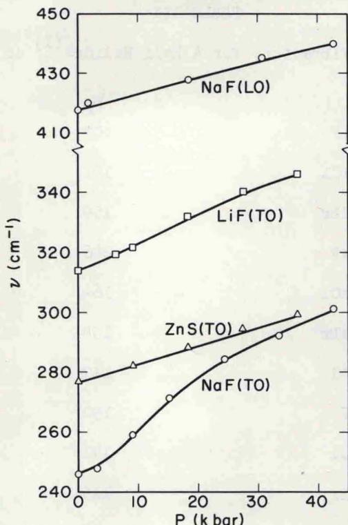
Fig. 1. Pressure Dependencies of Several Lattice Vibrations.
