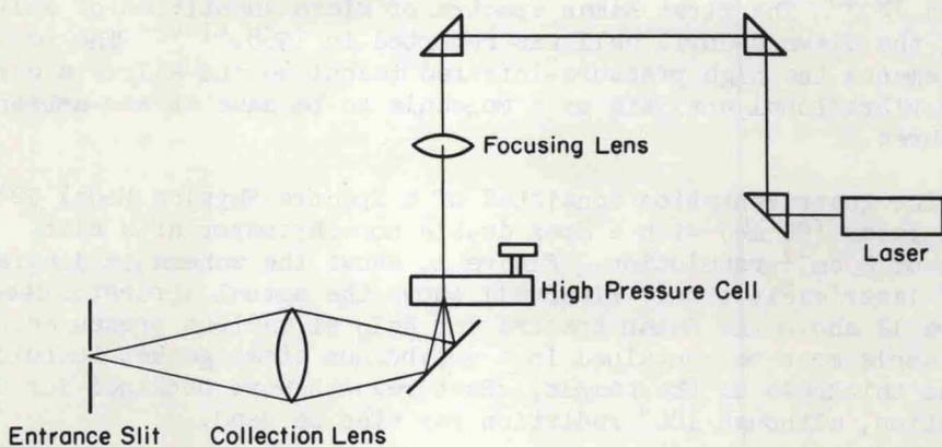
Fig. 10. Schematic Diagram for Laser Raman-High Pressure Experiment.
