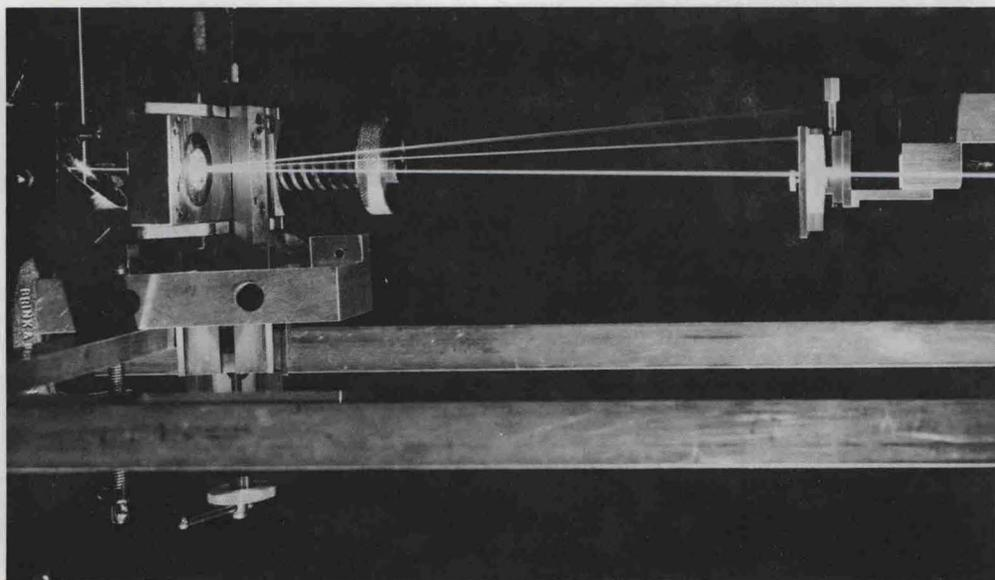
Fig. 11. Apparatus Used in Laser Raman-High Pressure Experiment.
